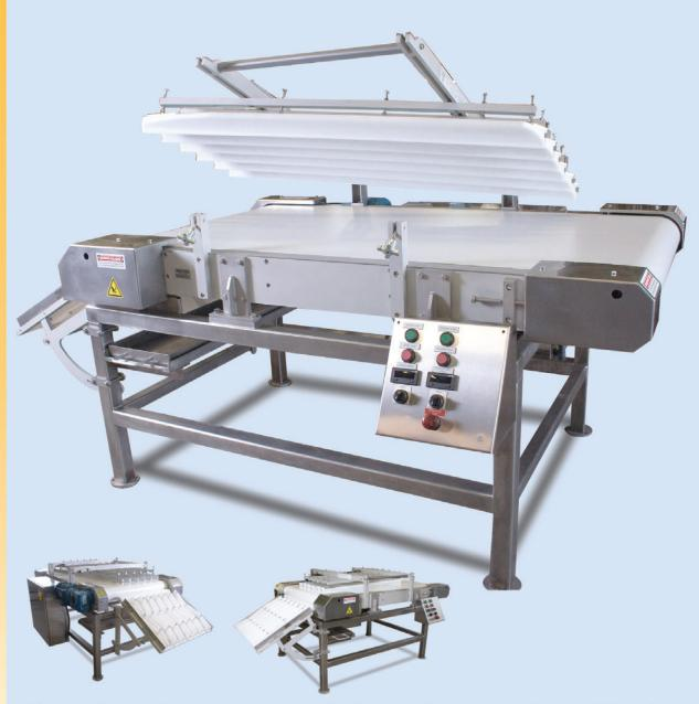
Machine Specialties knows good rounding is essential to bun production. Although many Rounder Beds look alike in appearance, performance can be radically different. Designed specifically for bun lines the Eagle Talon Rounding System has excellent consistent rounding incorporating a sanitary low maintenance design.
